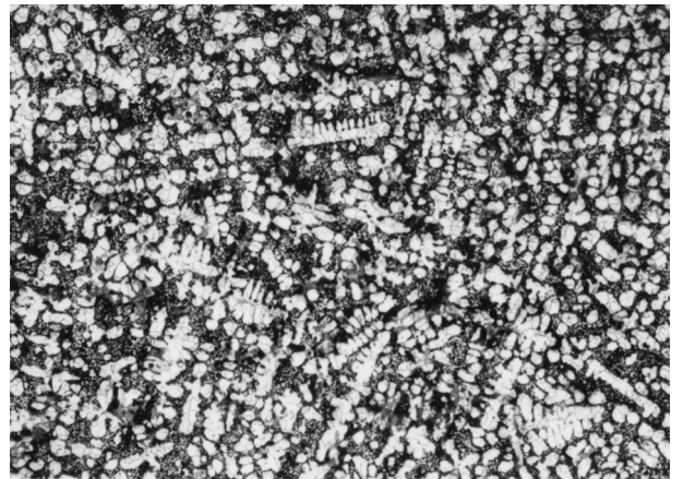
Figure 6 Photomicrograph of specimen E (cast with copper end chill). (Magnification, 1000 ×.)
