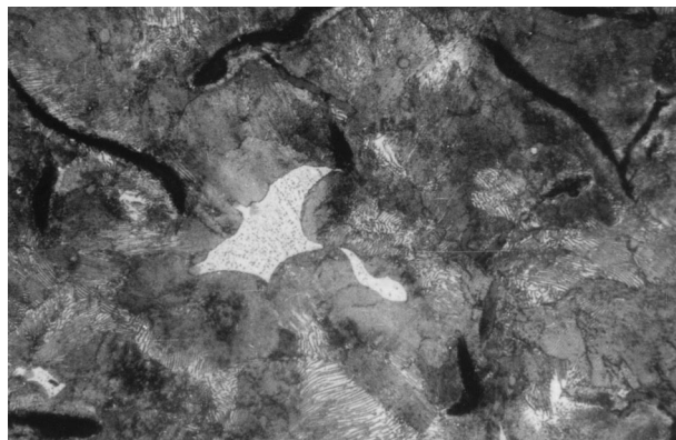
Figure 10 Microstructure of water-cooled chilled cast iron. (Magnification, 500×.)
