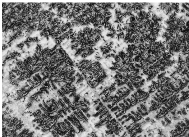
Figure 2 Photomicrograph of specimen A (cast with graphite end chill). (Magnification, 1000 \times .)
