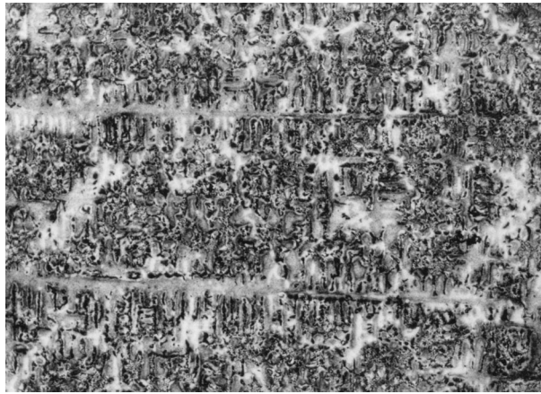
Figure 5 Photomicrograph of specimen D (cast with steel end chill). (Magnification, 1000 ×.)
